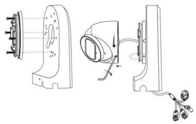
2 Waterproof the cable using the waterproof accessories that came with your camera, and use some tape to wrap the cables, then insert the cable into the box.
