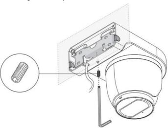
**Note:** When fixing the box to the bracket, make sure that the box is perpendicular to the wall and there is no gap between the box and the wall. Do not tighten the screw with too much force (do not exceed 10kgf.cm).
