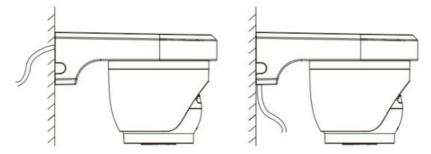
4Here we use the side exit for demonstration. After routing the cable, insert the provided silicone plugs to the other two outlets for waterproofing.
