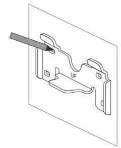
2 Drill four holes at the marked positions, insert the anchors into the holes, align the bracket to the anchors and drive the self-tapping screws into the anchors through the bracket.
