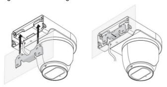
2 Secure the box to the bracket using the screw provided.
