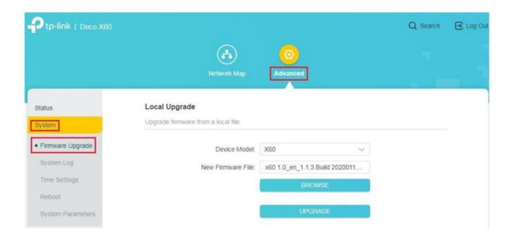
Step 5 Click the UPGRADE button. A small window showing "Uploading" will pop up, after the uploading, the next phase will be "Upgrading".
