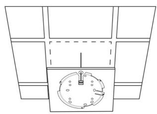
Connect the Ethernet cable to the Ethernet port. Please pay attention to the triangle sign. Attach the EAP to the mounting bracket, then rotate it until it locks into place, as shown on the left.
