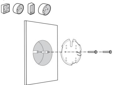
Route the cables through the square cable hole on the mounting bracket, and secure the mounting bracket to the junction box using screws. Then follow Step 4 and Step 5 of
