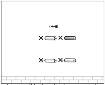
Secure the mounting bracket to the wall by driving the self-tapping screws into the anchors. Make sure that the shoulders of the mounting bracket are on the outside.
