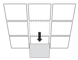
Place the mounting bracket in the center of the ceiling tile. Mark four positions for the screw holes and a location for the Ethernet cable hole. Drill four 4 mm (5/32 in) iameter holes for the screws and a 25 mm (63/64 in) diameter hole for the Ethernet cable at the marked positions.
