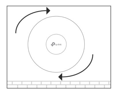
Attach the EAP to the mounting bracket by rotating it until it locks into place, as shown on the left.
