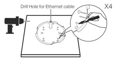
Secure the mounting bracket to the ceiling tile using four M3x30 pan-head screws, washers, and wing nuts, as shown on the left.
