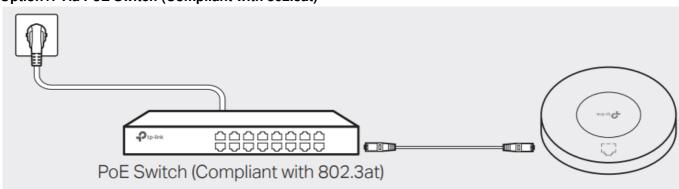
Connect an Ethernet cable from the PoE switch (compliant with 802.3at ) to the Ethernet port.
