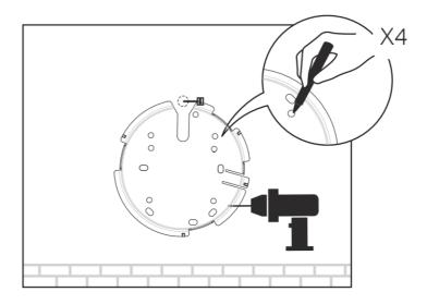
Insert the plastic wall anchors into the 6 mm diameter holes.
