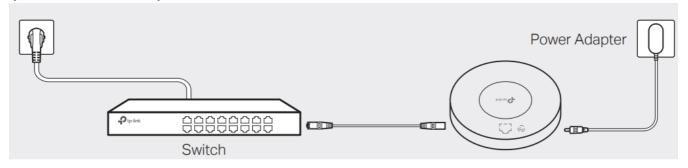
Plug one end of the provided power adapter into the power port of the EAP and the other end to a standard electrical wall outlet.
