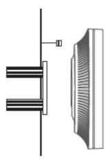
5. Attach the EAP to the mounting bracket, then rotate the EAP until it locks into place, as shown on the left.
