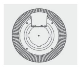
**RESET** With the device powered on, press and hold the button for about 5 seconds until the LED flashes quickly . Then release the button. The device will restore to factory default settings.
