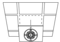
5. Connect the Ethernet cable to the Ethernet port. Attach the EAP to the mounting bracket, then rotate the EAP until it locks into place, as shown on the left.
