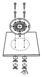
4. Feed the Ethernet cable through the hole and set the ceiling tile back into place.
