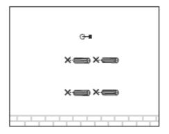
3. Secure the mounting bracket to the wall by driving the self-tapping screws into the anchors. Make sure that the shoulders of the mounting bracket are on the outside.
