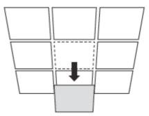
2. Place the mounting bracket in the center of the ceiling tile. Mark four positions for the screw holes and a position for the Ethernet cable hole. Drill four 4 mm diameter holes for the screws and a 25 mm diameter hole for the Ethernet cable at the marked positions
