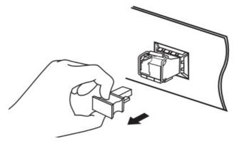
4. Plug a fiber-optic cable into the transceiver. Note that the transceiver works without any additional configuration
