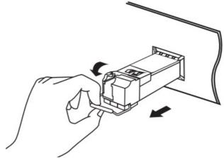
4. Reinstall the protective dust plug in the transceiver's optical bores and place it on an antistatic mat or a static shielding bag.
