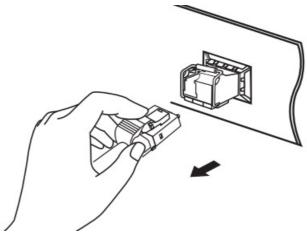
3. Pull the safety latch downwards to release the transceiver, and then pull it out from the slot
