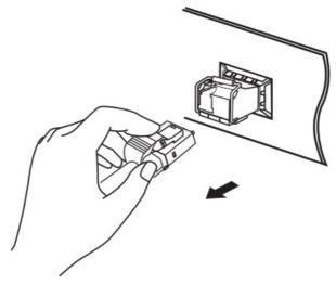
3. Pull the safety latch downwards to release the transceiver, and then pull it out from the slot.
