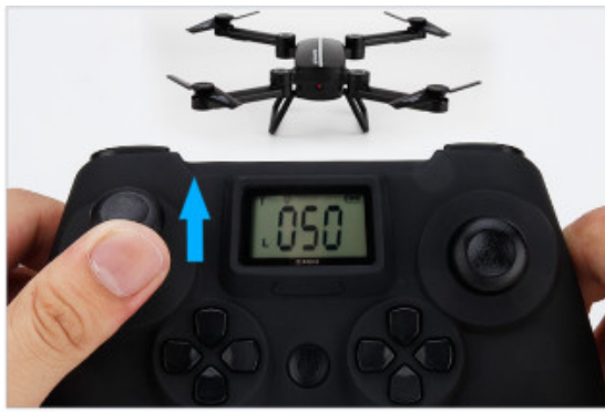
1: Push the throttle lever up
