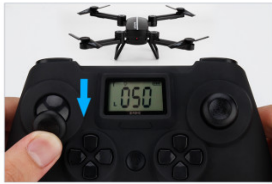
2: Push the throttle lever down
