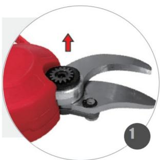
• PLACE THE OIL BOTTLE NOZZLE IN THE LUBRICATING PORT. HOLD THE OIL BOTT- LE UPRIGHT AND THEN LUBRIFIE;
