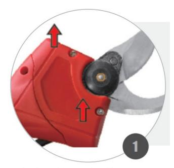
• USING THE OTHER TIP OF THE SPECIAL TOOL, REMOVE SCREW AND THE ELAS-TOMER WASHER;
