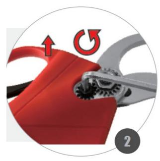
• AGAIN USING THE SPECIAL TOOL, REMOVE LOCKED SCREW NUT AND REMOVE RESISTANCE WASHER;
