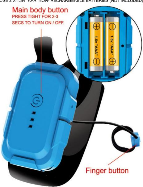
**GESTURE FUNCTION:** 1. SWING HAND BACK AND FORTH = CAR FORWARD/BACKWARD. 2. FINGER BUTTON + LEFT AND RIGHT SWING = CAR ROTATES LEFT AND RIGHT.
