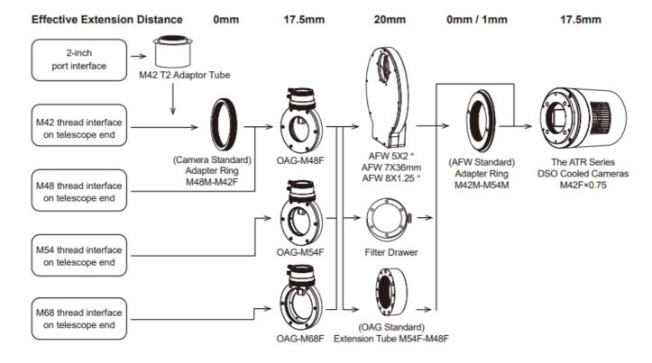
**Note:** When using ToupTek Astro accessories, screw connection is recommended for other brands of accessories, an adapter ring can also be used.
