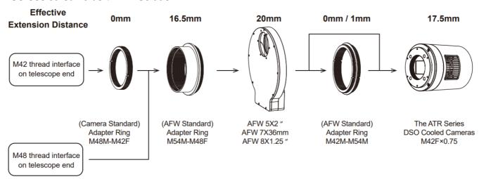
Note: Connecting to the telescope's M42 interface may cause obstruction to the camera's full frame.
