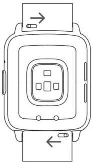
Slide the spring pin and hold it while pulling away from the watch to remove the current wristband. To attach a new band, slide the spring pin across and slot the new band. When both sides of the band are positioned correctly, release the spring pin.
