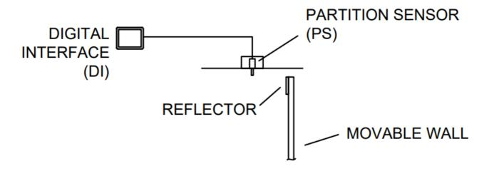
THE PARTITION SENSOR MUST BE IN LINE WITH THE REFLECTOR AND WITHIN 10' OR LESS.
