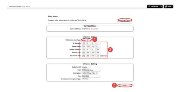
STEP-3.2.2: Advanced Setup Static IP setting
