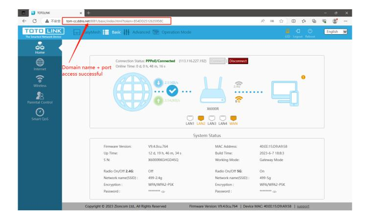
You can also ping the domain name through the CMD of the PC, and if the returned IP is a WAN port IP address, it indicates successful binding.
