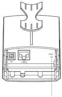
RESET Press the RESET button for about 8 seconds until the signal strength indicators blink.
