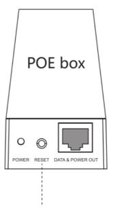
RESET on PoE box Press the RESET button on PoE box for about 8 seconds until the signal strength indicators blink.
