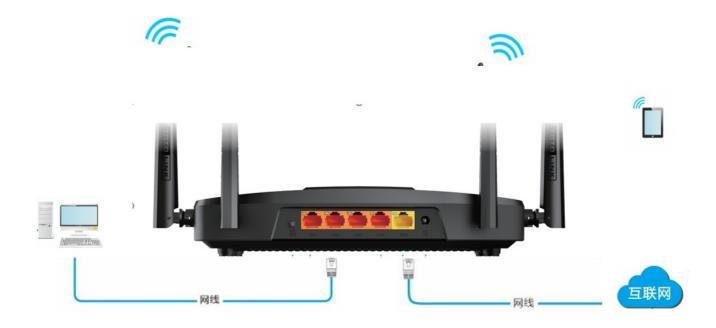
If you don't have a PC, you can also use your mobile phone or tablet to connect to the router' WiFi. The SSID is generally TOTOLINK\_model, and the login address is itotolink.net or 192.168.0.1
