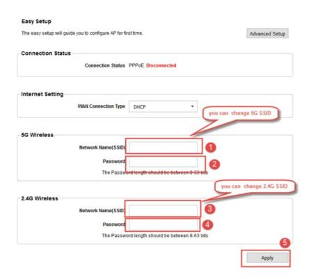
STEP-2: B-Router Repeater Setup
