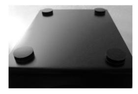
If the KIN Solo is placed on a surface, Totem recommends decoupling the loudspeaker with the supplied feet to break down cabinet resonance for optimum results. Turn the speaker upside down and apply the adhesive-backed feet to the 4 corners and middle of the cabinet.
