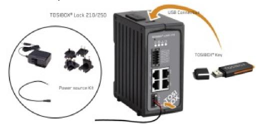
1. Connect the operating voltage of 12-48 V DC to the Lock and wait for 1 minute. In case you have a product version with a Power Source kit, use the conversion cable. It onverts the AC adapter's coaxial connector output to stripped wires that are needed to power the Lock 210/250. Follow the polarity symbols in the front panel. Use +
