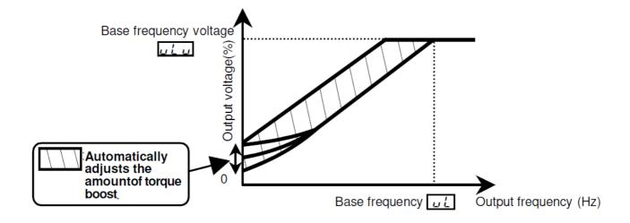
**Note:** This control system can oscillate and destabilize runs depending on the load. If that should happen, set V/F control mode selection PT to 0 (V/F constant) and increase torque manually.
