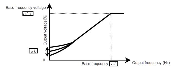
To increase the torque further, increase the setting value of the manual torque boost .
