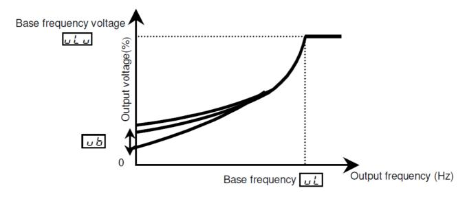
3. 3) Increasing starting torque Setting of V/F control mode selection PT to 2 (automatic torque boost control)
