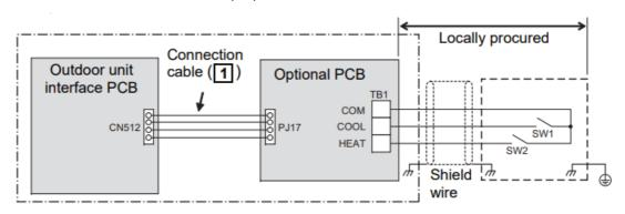
**SW1:** Cooling mode specified input switch **SW2:** Heating mode specified input switch
