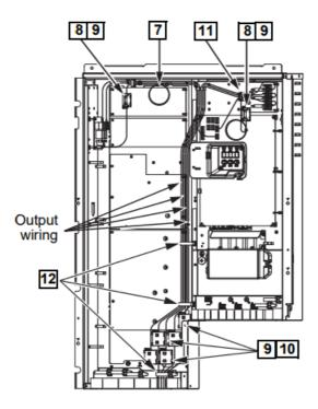
1. Attach the clamp filter (8) to the connection cable (1 or 2) and attach the clamp filter (10) to the output wiring
