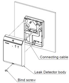
When mount Leak Detector body to rear cover, take care not to pinch connecting cable among body and rear cover.
