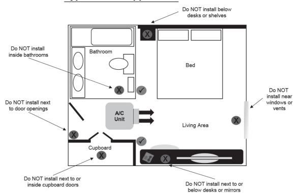
You need to observe the regulations of the local governments, state and country that govern the installation of Leak Detector when installing the Leak Detector. You must ensure that installation complies with all relevant rules and regulations.
