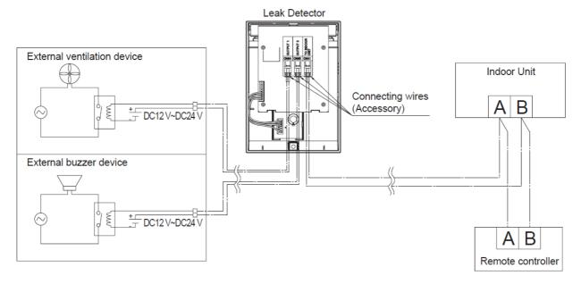
Output connector can be connected the external device (Ventilation, external buzzer device and etc.) When the Leak Detector detects leakage, outputs the signal to these device. When the buzzer is stopped, Output 1(CN64) will keep to output, Output 2(CN65) will stop to output.
