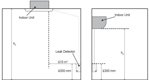
It must be placed within a horizontal distance of 10 meters and on the wall in the room where the indoor unit is installed. However, when it does not enter the field of view on a straight line from the Leak Detector, it is within 7 meters at the shortest horizontal distance without obstacles and installed on the wall in the room where the indoor unit is installed.
