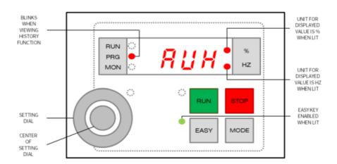
1. The panel frequency command is accessed by adjusting the setting dial while in Standard Mode. When saving a change, the display will flash FC.
