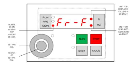
The output current is displayed in units of % by default. This is a percentage of the VFD's output current rating. Typically, it is more helpful to read this number directly in units of Amps. Setting parameter f701 to 1: A(ampere), V(volt) changes the unit from % to A.
