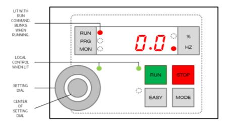
Standard Mode displays the Output Frequency in the main window by default. This can be programmed to other monitor items via parameter f710. Section 1.3 of the S15 Instruction Manual E6582175 provides fur-ther details.
