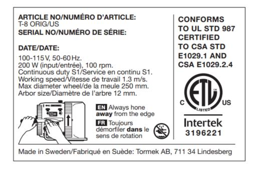
**WARNING** Read the instructions before operating the machine. Do not use in area where children may be present. Do not make adjustments until the wheel has stopped running. Wear eye protection. Use grinding wheel suitable for 150 RPM.
