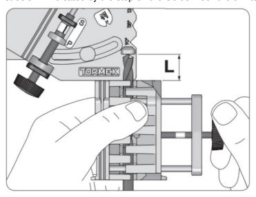
• Loosen the wheel and rotate the drill so that the cutting edges are aligned parallel to the horizontal lines on the Drill Holder. Tighten the wheel. The protrusion L does not need to remain exact.
