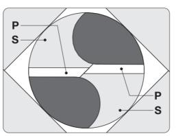
Feed the nut S a bit further. Try with  $\frac{1}{4}$  of a turn. One turn is equal to 0.5 mm (0.02").
