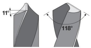
• The clearance angle. Place the Setting Template according to the image and tilt the base (1) so that the corners of the Setting Template touch the grindstone. Lock it securely with the wheel (6).
