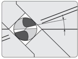
• The drill is mounted correctly. The width of the primary facets is even.
