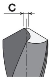
More expensive drill bits are ground with special points of various types. These drills must be re-sharpened in their original production machines or in special machines, which are available only at a few specialist sharpening shops. They can also be re-shaped to a 4-facet point with the Tormek attachment.
