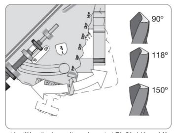
• The clearance angle ( $\alpha$ ) is set by tilting the base. It can be set at 7°, 9°, 11°, or 14°.
