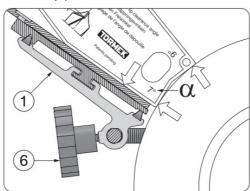
• The point angle. Measure the existing point angle in the grooves on the Guide or select the angle that is most
