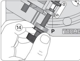
• Press the drill holder towards the grindstone and grind one of the primary facets. Move the guide back and forth across the grindstone.
