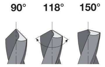
Centering drills usually have a 90° point angle. A drill bit needs to have the right lip clearance angle to cut the material. The clearance angle varies from 7° to 14°. A drill with a larger clearance angle cuts more easily, but if the angle is too large, vibrations will occur and the drill will cut irregularly and quickly become dull. If the clearance angle is too small, the drill will not cut at all, but will become hot and rapidly destroyed.
