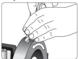
The flute is honed on one of the profiled leather honing wheels. Select the wheel according to the size of the drill.
