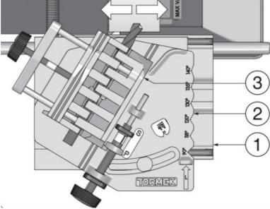
• The high precision drill holder consists of two identical parts. The drill will be exactly centered, and both of the cutting edges will be sharpened exactly to the same shape.
