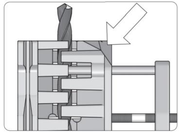
• Mount the drill with the protrusion L indicated by the stop on the Guide. Lock the drill temporarily
