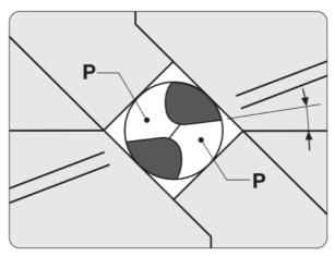
• When the grinding is finished, the primary facets P should be parallel to the horizontal line.
