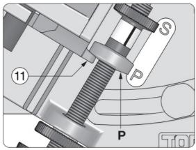
• Lift and turn the drill holder 180° and grind the other primary facet in the same way
