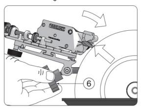
• Screw the stop nut S forwards. Start with 1½ turns for a 6 mm (¼") drill. The setting screw should still be locked with the locking nut (14).
