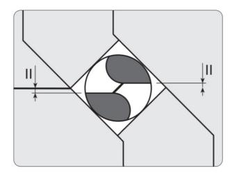
**Note:** Here, it is shown how to mount and grind a slightly blunt drill. Heavily worn and broken drills need a different setting in the Drill Holder. This is because the direction of the cutting edges changes gradually during the grinding. See page 13.
