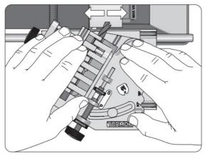
• You can tell by the decreasing sound when the primary facets P are ground equally. How far they are grounded over the centre does not matter. They must be grounded symmetrically. The primary facets should meet and form a flat chisel edge, C.
