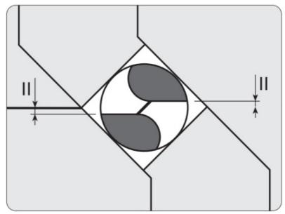
• The grinding depth for the first two facets is determined by adjusting a setting screw which has a stop, P. These initial facets are called primary facets.
