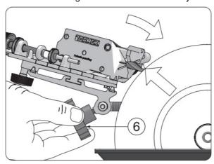
• Turn the setting screw (13) lightly towards the grindstone and grind carefully until the 4-facet point is established again.
