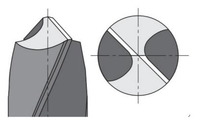
All the components are made with high precision which ensures that the lengths of the two cutting edges will be equal within close tolerances. This is an essential requirement so that the two edges will work in the same way and so that the drill will bore a round, straight hole, which is not larger than the drill diameter.
