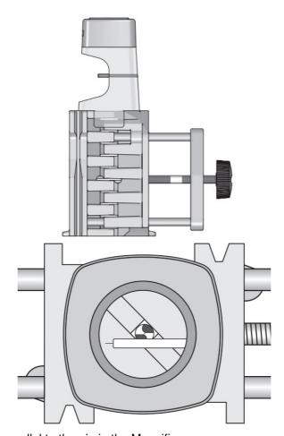
The cutting edges should be parallel to the pin in the Magnifier
