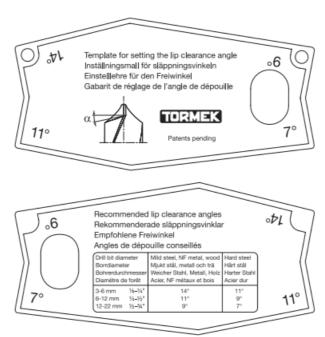
Clearance angle. With the Tormek Setting Template you can set the clearance angleto 7°, 9°, 11° or 14°. The Template recommends a suitable angle based upon the drill size and the material to be drilled.
