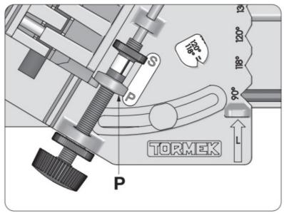
• After grinding one facet, the drill holder is turned 18,0° and the other facet is ground to an identical shape. Now both of the two primary facets are grounded.
