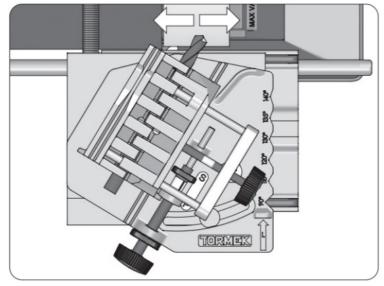
• After grinding the primary facets, the drill holder is moved forward to a second stop S for grinding the secondary facets, which gives the drill a 4-facet point.
