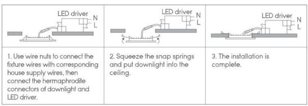
According to the three steps as showing in above pictures. please refer for the above specification list tor cutout size. Please make sure the correct cutout size in order to make the light ix well within the ceiling and have no risk of falling of.
