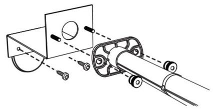
Fig. 2 Attach lamp to lamp bracked and install in desired location.
