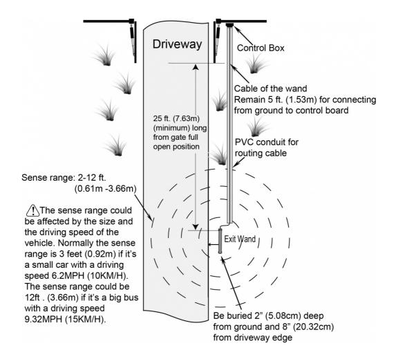
NOTE: Keep the WAND and the cable uncovered before the function has been tested OK.
