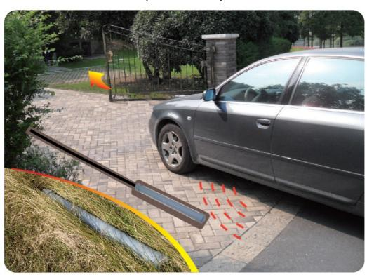
NOTE: The exit wand may be activated automatically in a strong magnetic field or be activated by coins, tools, or any other metal objects if the selectivity is set too high. You may decrease the sensitivity by adjusting the sensitivity board towards the anti-clock direction or even pull the sensitivity board directly off. Please make sure the sensitivity is set at a proper level and find a suitable position before burying it.
