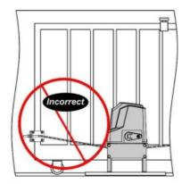
Make sure there is 1" distance at least between the wheel cover and the gate after you position the base plate.
