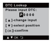
After you input the DTC, press [OK] to view its detailed definition.
