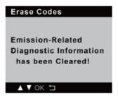
**Note**: Be sure the vehicle's ignition key is in the ON position with the engine off.
