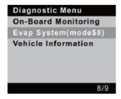
If the vehicle doesn't support mode\$8, the following result will be displayed on screen.
