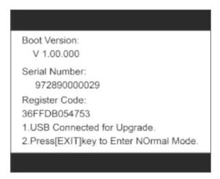
• Press [EXIT], and enter the main menu. Run the Update Tool in your computer. The system will automatically detect the Serial Number of the scanner. Select [Print Manager].
