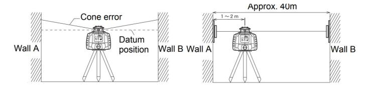
Perform the following check after completing horizontal calibration procedure.
