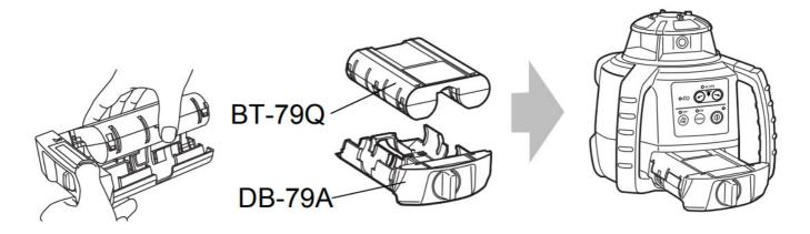
RL-H5A (Using the dry cell batteries)
