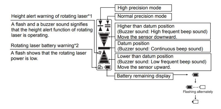
**Note:** The warning displays \*1 and \*2 are the functions that the level sensor detects alarm signal from the rotating laser.
