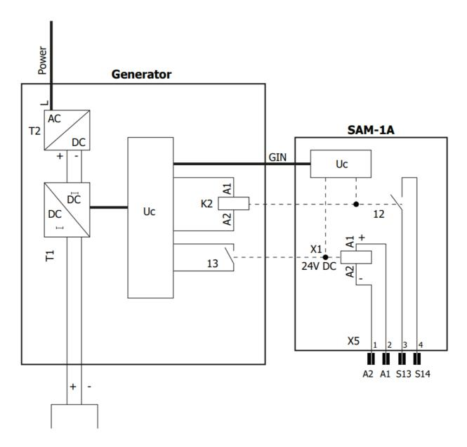
5. Electrical characteristics of terminal block X5 inputs/outputs
