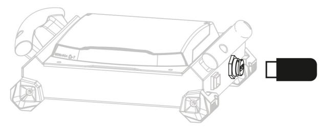
3. The screen comes on if a new software version is detected. Wait until the step is complete and restart the product after having disconnected the USB key.
