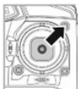
Right Joystick Lower Arm with Bucket Tilting Down
