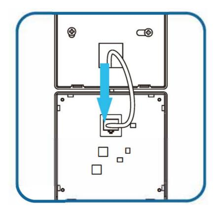
Inserting CAT-5 cable to control board, a clicking sound indicates the successful connection.
