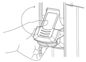
3. insert the power cord plug into the external connector of the charging trolley, press down the silver slider, and with it pointing upwards. Then turn the plug to the right until the slider clicks into place and connect the other end with the AC socket.
