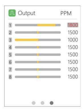
In the PPM output page, press down on the roller for 2 seconds to set the output value of each channel.
