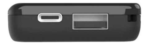
Press and hold [Wheel] 2 seconds to enter the setting menu, you can set the USB cutoff voltage. When the battery discharges past the set value, the MC8 will disable both USB-A and USB-C output; the buzzer will also give an extended tone, indicating the protection voltage has been reached.
