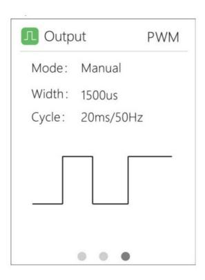
**Mode** Signal output mode- can be changed between manual and 3 automatic modes of varying speeds.
