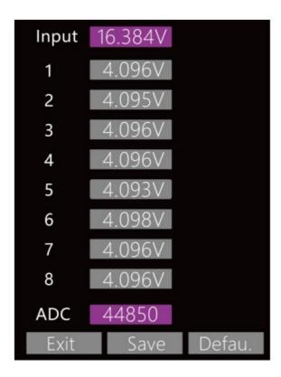
Measure the voltage of a fully-charged battery pack using a multimeter. Use the roller to select Input, then scroll until the value matches what was measured on the multimeter. Scroll down to save and press down on the roller to save. Repeat this process for each individual cell if needed. When finished, scroll to the exit option and press down on the roller to finish the calibration.
