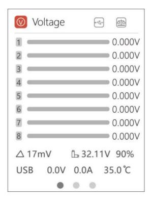
1. The MC8 displays the total voltage of all battery chemistries operating within the input limits .
