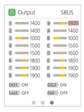
In the SBUS output page, press down on the roller for 2 seconds to set the output value of each channel.
