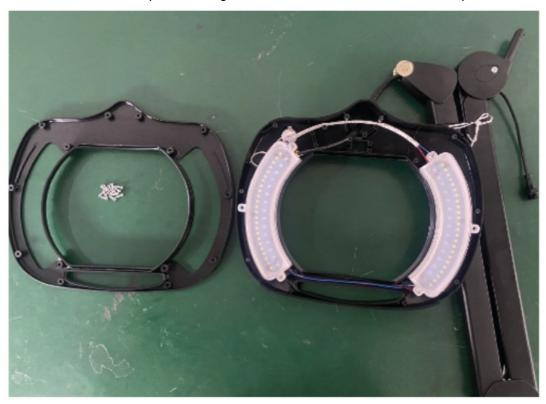
**Step 3**Pull out the wire from the arm and disorder the PCB in the lamp head.
