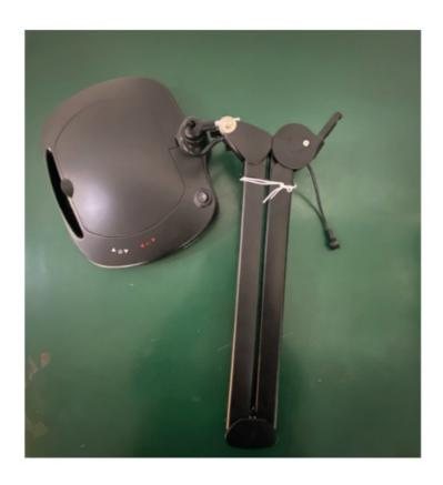
**Step 2**Use the screwdriver to remove the screws from the metal connector. Take out the knob, use the soldering to disorder the wire and separate the light source with the arm. Pull out the lamp cover.
