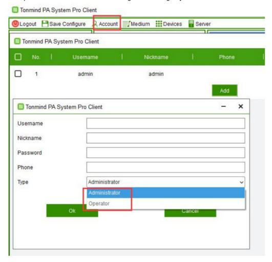
All IP audio endpoints to be connected to Tonmind PA System Pro support SIP protocol, and each of them needs to be configured with a SIP account.
