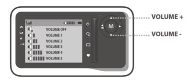
Press ▲ UP to increase or ▼ DOWN to decrease the volume of the parent unit. Mute icon will be displayed if the volume is turned off on the parent unit.
