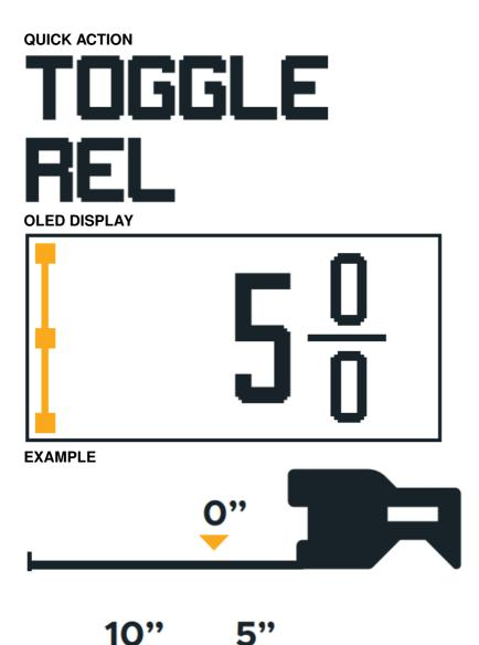
**NOTE:** To confirm that you are using the TOGGLE RELATIVE Quick Action, look for the bracket on the left side of the OLED Display
