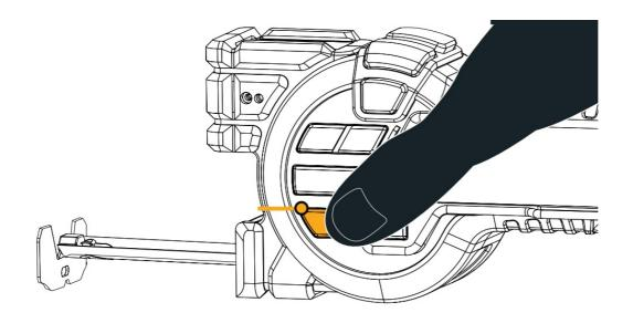
**STEP 3**PRESS CAPTURE BUTTON TO SAVE MEASUREMENT TO E-PAPER DISPLAY
