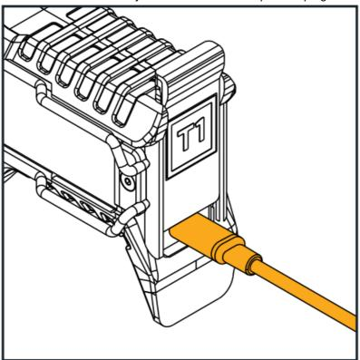
STEP 3: Once fully charged, unplug the USB-C cable and slide down the Battery Lid to securely close it.
