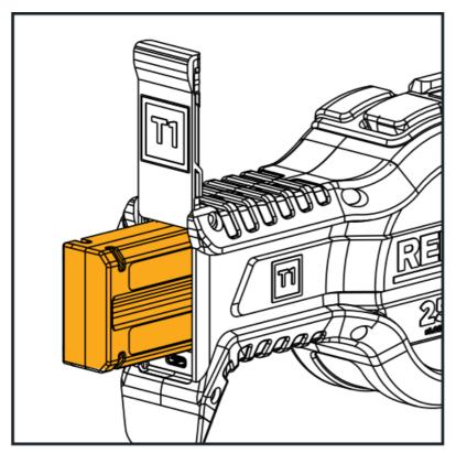
STEP 2: Slide the Battery Lid down and leave space to plug in USB-C cable into the provided USB-C port.
