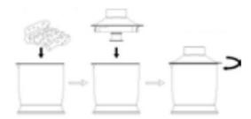
**Caution:** do not switch on the mincer constantly, this could cause problems with the motor. Preferably use the mincer one minute each time and then allow the motor unit to cool down for one or two minutes.
