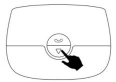
4. Tear off the insulation film on the battery, then put back the battery to make the equipment electrified. Now the device is in a configuration state, close the back cover
