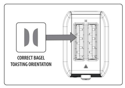
IMPORTANT: If using BAGEL function, ensure the cut side of the bagel faces the outer heating element of the
