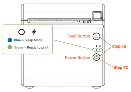
After configuring your Toast Printer, the LED will be blue if the printer is in Sleep mode. This happens if the printer is turned off or unplugged. To power it back on, hold the Power button until the LED turns green.
