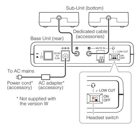
Note When using a headset, set the Base Unit's headset switch to ON.
