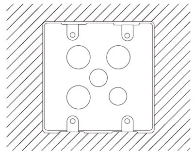
2. Connect CAT5-STP cable, then install the panel into the 2 gang box and tighten it with accessory screws.
