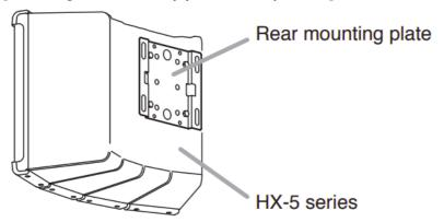
Use the rear mounting plate with its orientation pre-fixed at the factory
