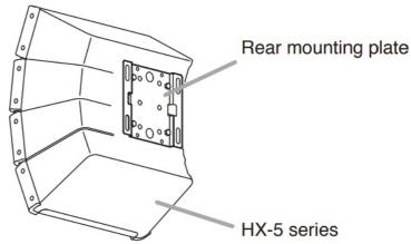
[Mounting to vertically-positioned speakers]
