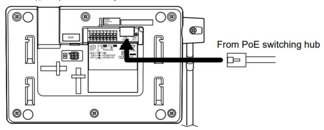
Compatible switching hubs: Switching hubs conforming to PoE (IEEE802.3af Class 3) specifications
