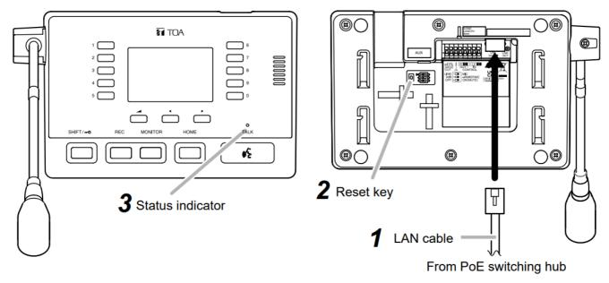
Step 1. Connect the IP Remote Microphone to the PoE switching hub using a LAN cable.
