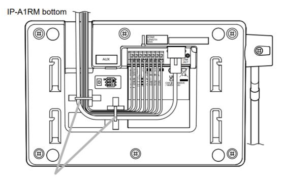
Bundle the cables and secure them to the fixing holes for wiring with the zip ties supplied with the IP-A1RM.
